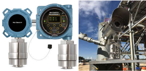
Figure 16: Fixed point combustibles and toxic gas detectors use multiple sensor technologies, such as infrared, catalytic bead and electrochemical. The Net Safety Millennium II series (left) can detect all flammable gases and common toxic gases. Rosemount 935/936 Open Path Combustible and Toxic Gas Detectors (right) use infrared and ultraviolet technology to detect hydrocarbon and toxic gases, including methane, propane, ethylene, hydrogen sulfide and ammonia.
